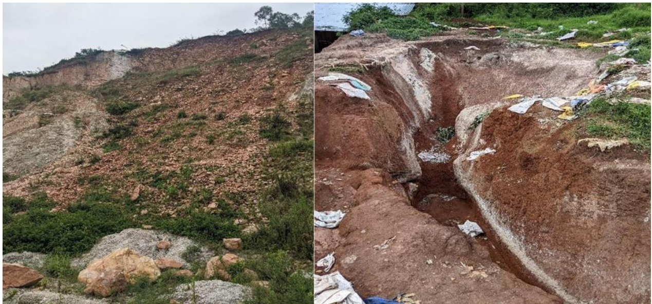
Figure 4.4 : Exposed tailing dams in MMB which are not well managed
